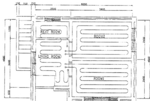
Fig. 1 Schematic of the panel heating system.
