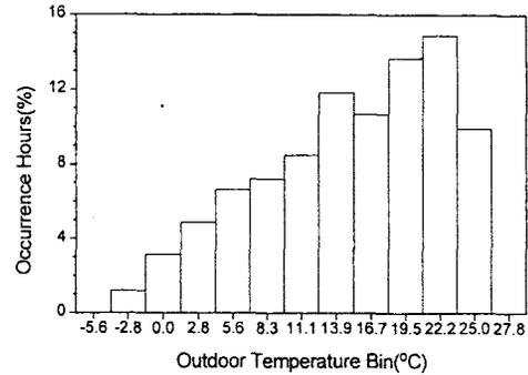
Fig. 4 Occurrence hours as a function of outdoor temperature bin during the test period from March to June.
