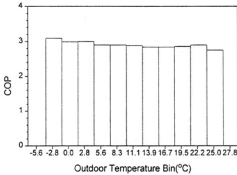
Fig. 6 Averaged COP as a function of outdoor temperature bin during the test period from March to June.
