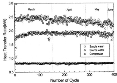
Fig. 8 Variation of heat transfer rate and power input during the test period from March to June.
