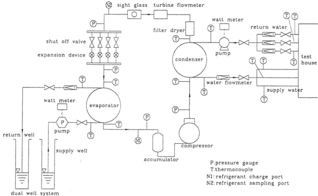
Fig. 3 Schematic diagram of the water-to-water heat pump system.
